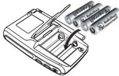
**Caution:** Installing batteries incorrectly can damage the TV.
